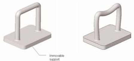
Figure 13 A firmly supported bracket can't move without deformation.
